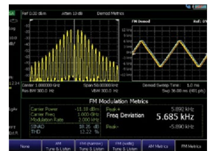
Characterize AM/FM signals using AM/FM demodulation
