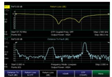
View return loss and DTF simultaneously
