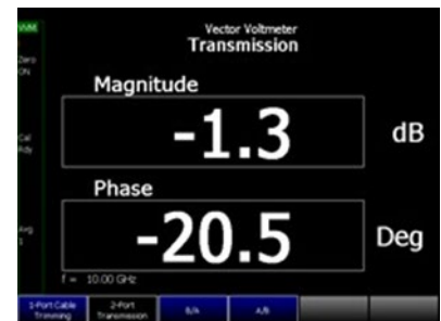
Simplify cable trimming with the vector voltmeter capability
