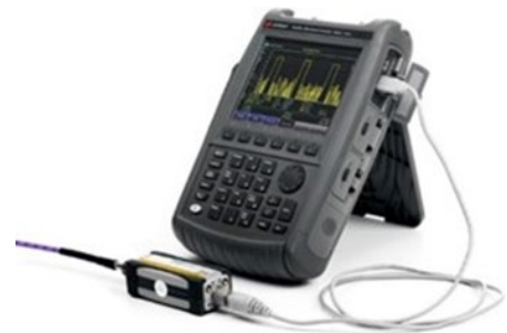
Simplify power measurements with USB power sensors
